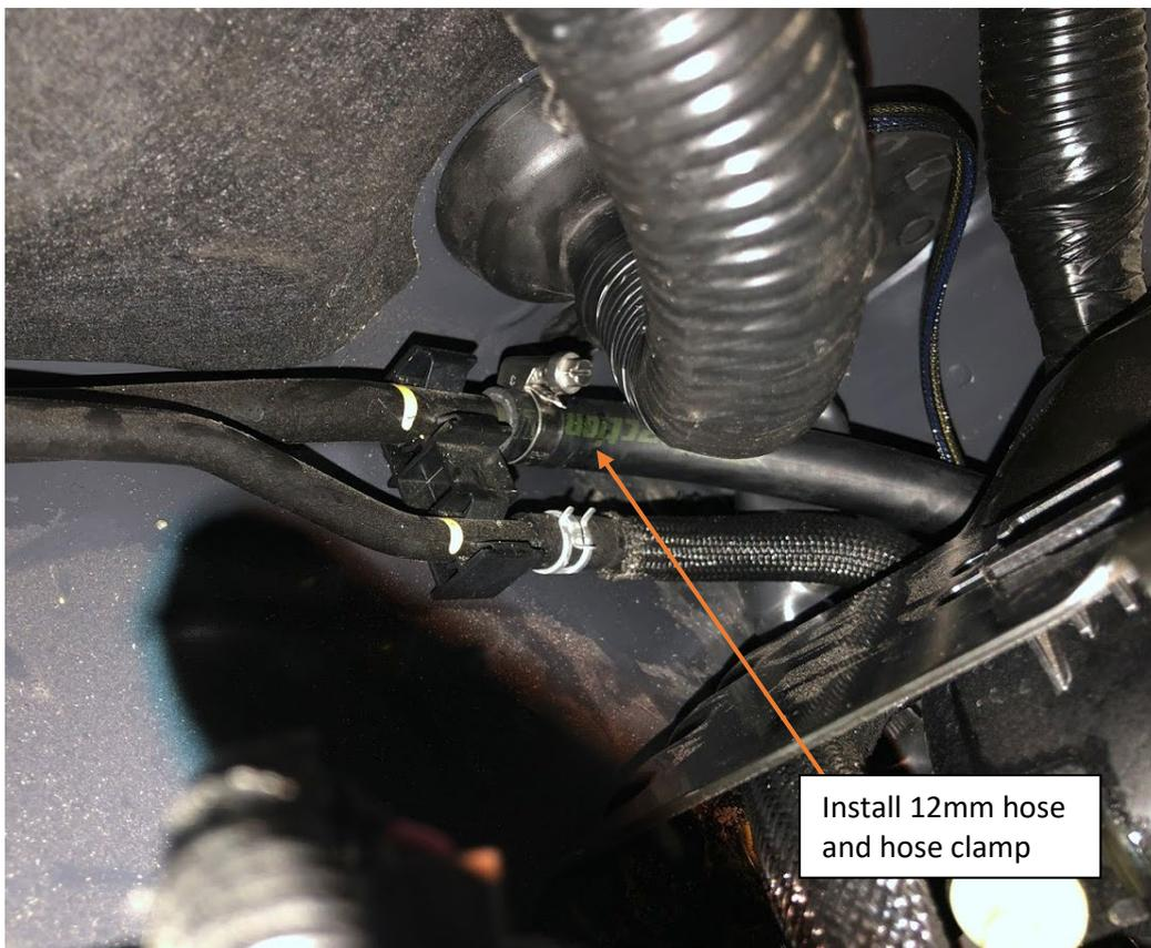
7. Route the 12mm fuel hose around the factory filter and down the inner guard to the Inlet port of the Prefilter.
